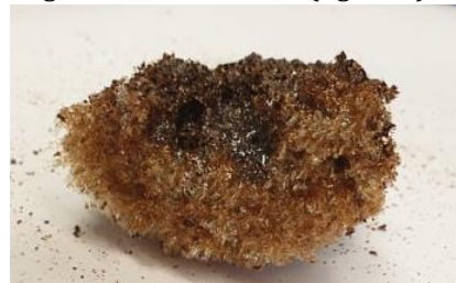
Figure 3 - Microwave-cured polyglycerol citrate/sawdust.
