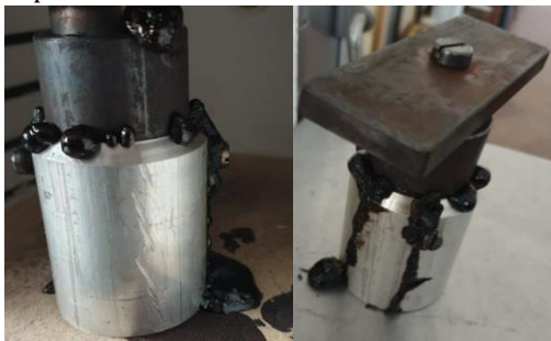
Figure 11 - Sawdust/ Corn Starch/ Glycerine composite after the test in which it was found to be a thermoplastic.
