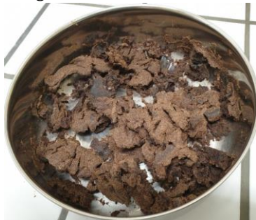
Figure 5 - Glycerine/ corn starch/ sawdust after curing in the oven.
