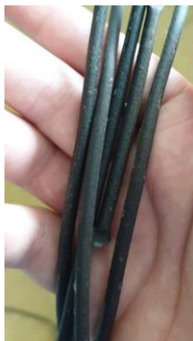
Figure 13 - Filament obtained using the 4-mm nozzle.
