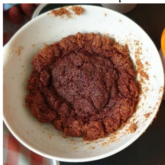
Figure 2 - 2:1 Polymer with sawdust, microwave cured.
