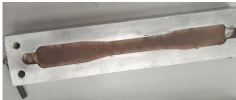
Figure 7 - Specimen for tensile test after curing in the oven for 12 hours at 140/150°C. Composite with 16.67% of sawdust by mass was used.
