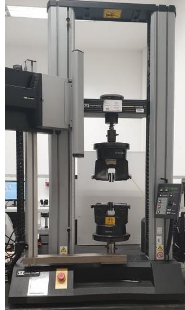
Figure 12 - The Instron 5566 Universal Testing Machine, used to perform all of the mechanical tests.
