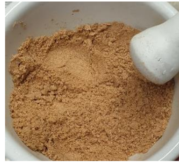
Figure 6 - Corn-starch/ glycerine/ sawdust composite prepared in the mortar, before being deposited in the dies.
