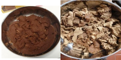
Figure 4 - Pre-polymer with wood, before drying in the oven. In the first image, the viscous solution is fresh off the hotplate and in the next one after 1 hour in ambient air.
