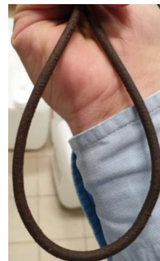
Figure 14 - Filament obtained using the 3-mm nozzle.
