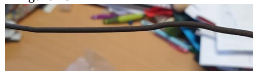
Figure 15 - Filament achieved using the 2-mm nozzle.
